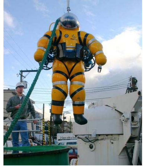
Specialized atmospheric diving suits used to conduct the underwater diving operation
