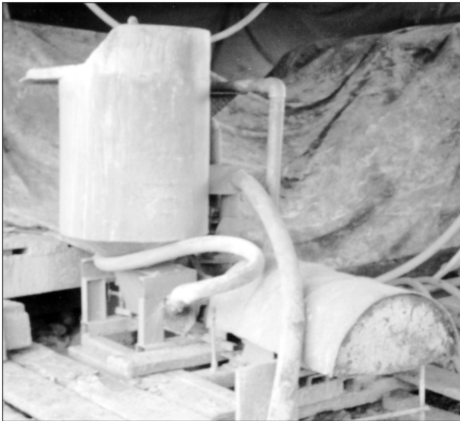
FIGURE 10 - COLLOIDAL GROUT MIXER
