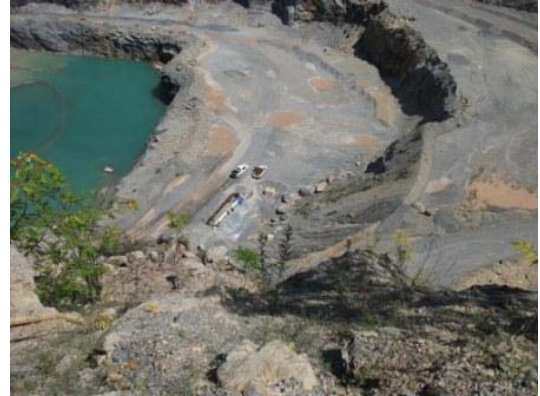
Pipes were set-up at the bottom of a quarry to test the effective delivery of the grout even when the equipment was located over 70 m higher than the point of injection
